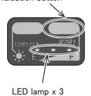
LED lamp lighting condition Contents of indication Left Center Right Remaining battery power of Lit Lit Lit 100 to 70% Remaining battery power of Lit Lit 70 to 30% Remaining battery power of Lit below 30% Blinking No battery power remaining \*1 Battery pack unattached \*2 Blinking Safety device activation \*1 Blinking
